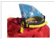
Provides effective protection of the face and forehead area of the injured. To be applied at rescue bag with the corresponding velcro/bracket mounting. Collapsible for easy and fast access. Transparent and cold-resistant foil material with Delrin battens.
