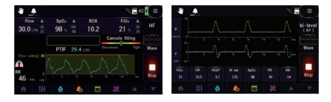
\*Volume guarantee? This function is to convert the target from pressure to volume during inspiration. It can be applied in spontaneous(S), spontaneous / timed(S/T), timed(T) modes, and replaces the inspiration target set value with the tidal volume from the inspiratory positive airway pressure. The provision of tidal volume is limited only by the pressure limit set. Set range: Off, On
